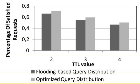
The optimized distribution process reduces the number of distributed queries (figure on the left). This, in its turn, reduces the wireless channel congestion and increases the reliability of the data distribution process (figure on the right).
