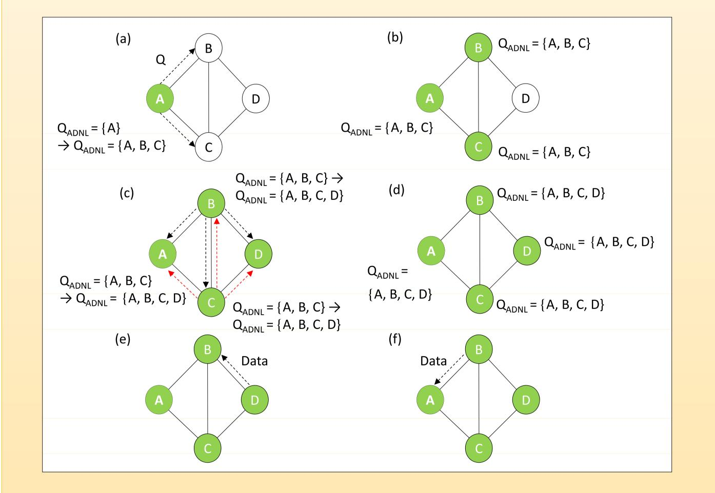
RECOWER context distribution is based on **context queries**. Context queries are distributed by using a one-hop broadcast-based approach, while context data are routed by using a unicast-based approach. If node D produces context data node A is interested in, the context distribution in above figure can be summarized as follows:
