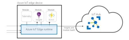
The runtime manages deployment and update of the modules, availability of the services reporting the status to the cloud and communication both with the cloud and the downstream to the devices
