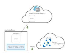
After the creation of the hub and the installation of the runtime, we want to deploy remotely the module from Azure portal to the loT device
