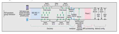
After the discovery phase, if a P2P device recognizes to have formed a persistent group with the corresponding peer in the past
