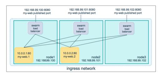
The overlay network *webnet* is load-balanced by using a round-robin strategy.
